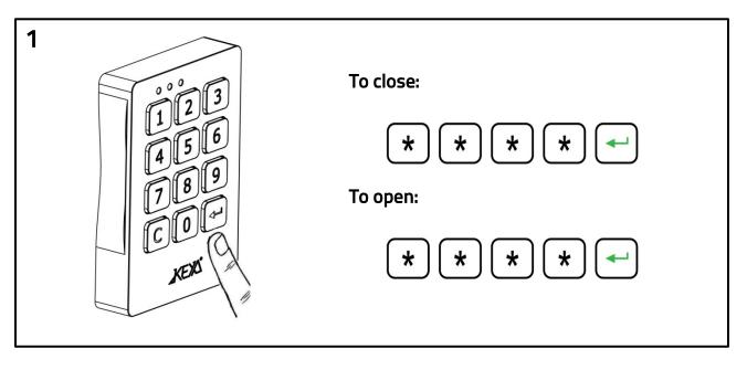
Open and close by 4-digit code. The code is erased every time the lock is opened, being available for a new use.
