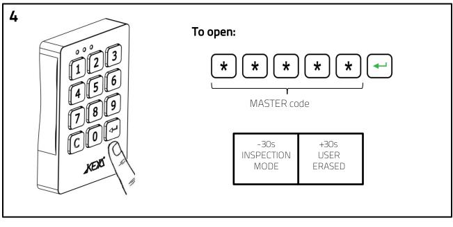
INSPECTION MODE Introduce the 5 digit Master code and press Enter Close the lock by pressing Enter before 30s. The User code is not deleted. DELETE USER CODE
