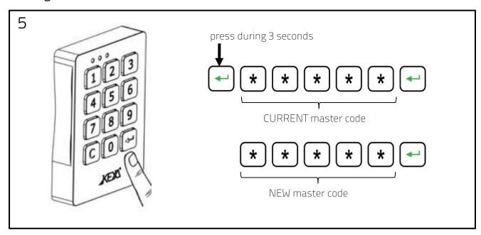
Press Enter during 3 seconds. Introduce Current master code and press Enter. Introduce New master code and press Enter.
