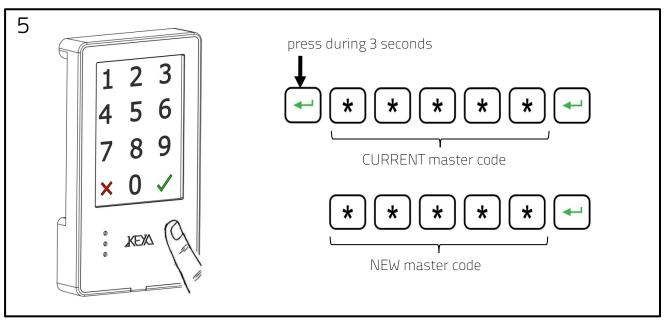
Press Enter during 3 seconds. Introduce Current master code and press Enter. Introduce New master code and press Enter
