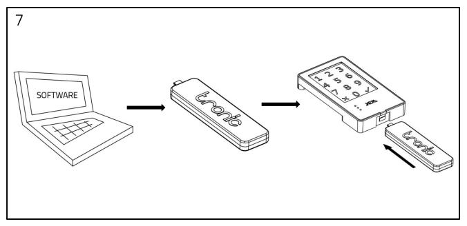
Load settings from the computer to the settings key. Connect settings key to the lock. The settings will be loaded into the lock.
