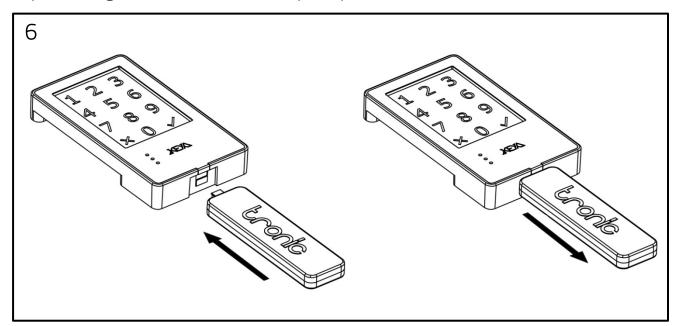
INSPECTION MODE Connect the Master key (BLUE) Lock opens Remove electronic key Press enter before 30 seconds User code is not deleted. DELETE USER CODE Connect the Master key (BLUE). Lock opens Remove electronic key After 30 seconds the User code will be deleted . A new User code will be required to close the lock again. AUTOMATIC OPENING TIME:
